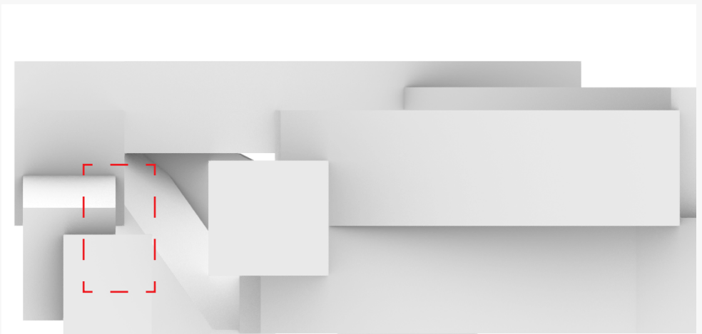
Choosing the intersection of 3 boxes with sloped surfaces for a representative chunk model
